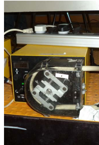
Figure 9: A peristaltic pump
