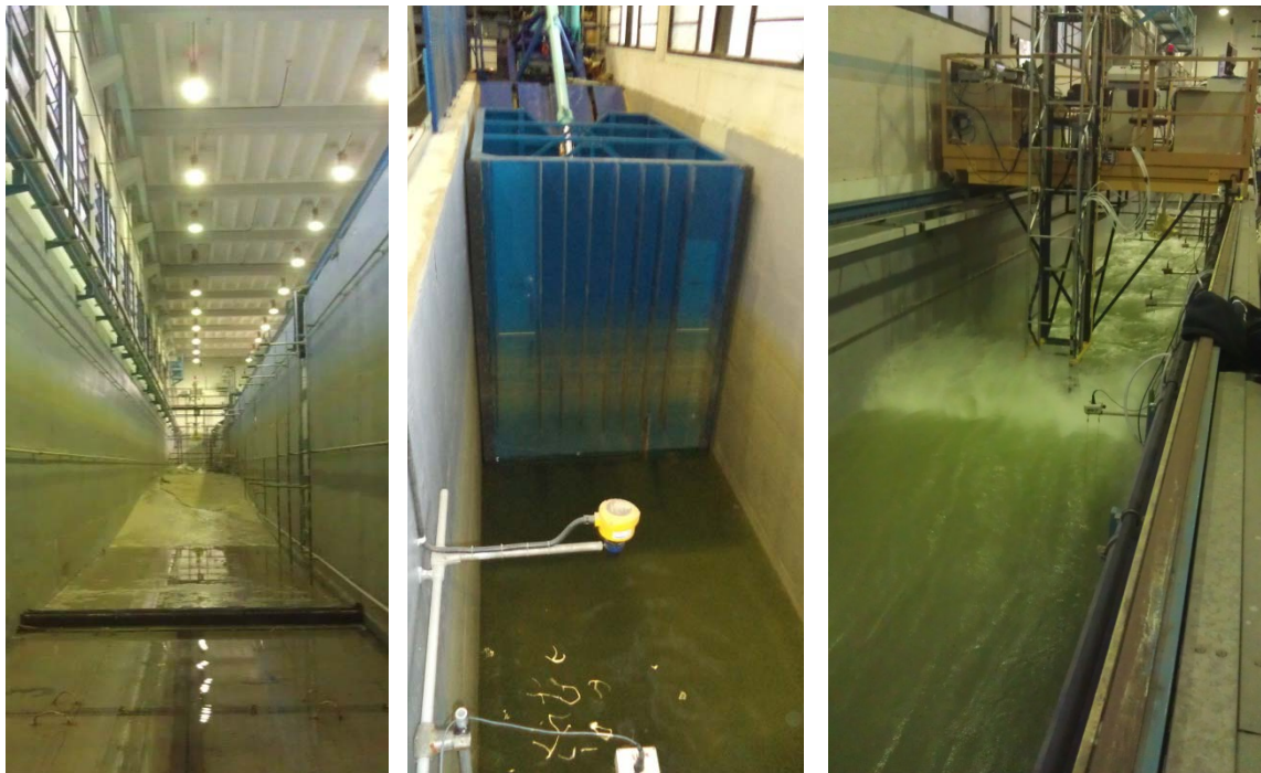
Figure 2: Three pictures of the CIEM wave flume in Barcelona: a) the empty flume with the counterfeit beach b) the wave paddle that generates waves and c) the measuring of plunging waves
